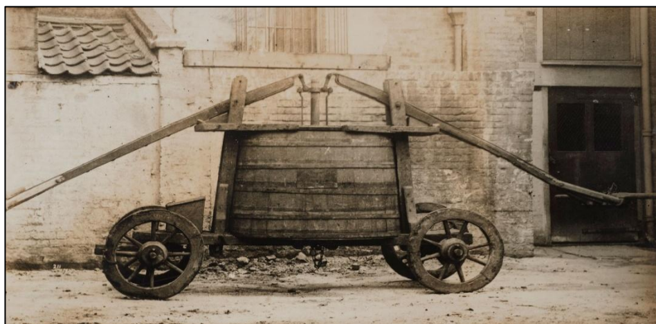
A seventeenth century fire engine, of the type purchased for Windsor in 1681
