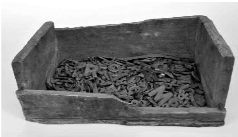
Typeset letters and numbers used as patterns at Hedges Foundry, Bucklebury. MERL 2006/47/11.
